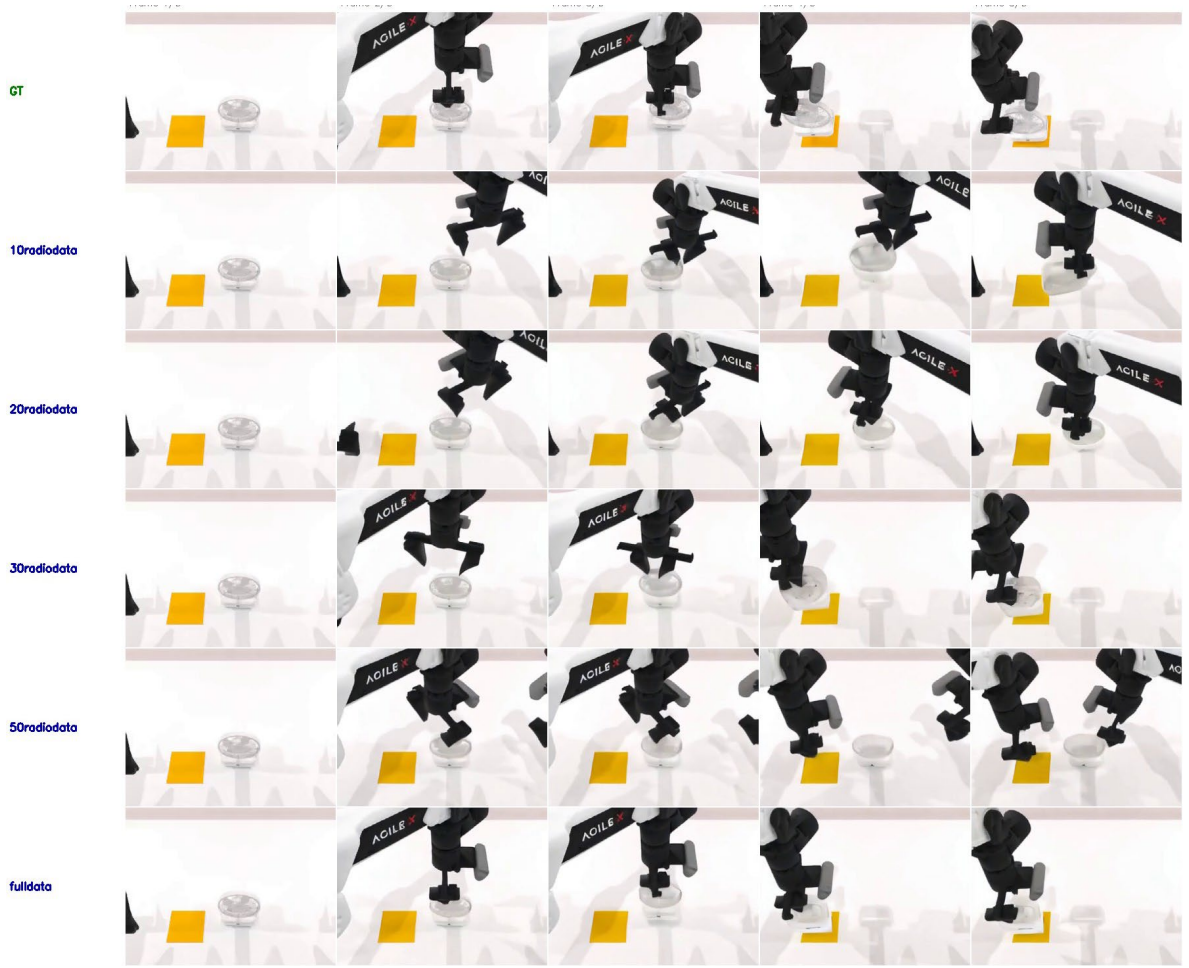
Figure 6: Qualitative evaluation of world model rollouts: We compare the keyframe sequences generated by policies trained on varying data scales (10% to 100%) against the GT. These sequences are used as visual prompts for both VLM-based and human-based success evaluation.
